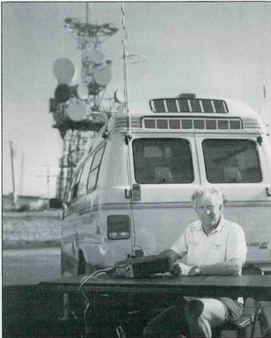
Gordon tests a 154-MHz Par notch filter right under a powerful pager site near Los Angeles. The filter did its job well!
