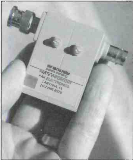
This small Par Electronics notch filter fits directly on top of a handheld scanner.
