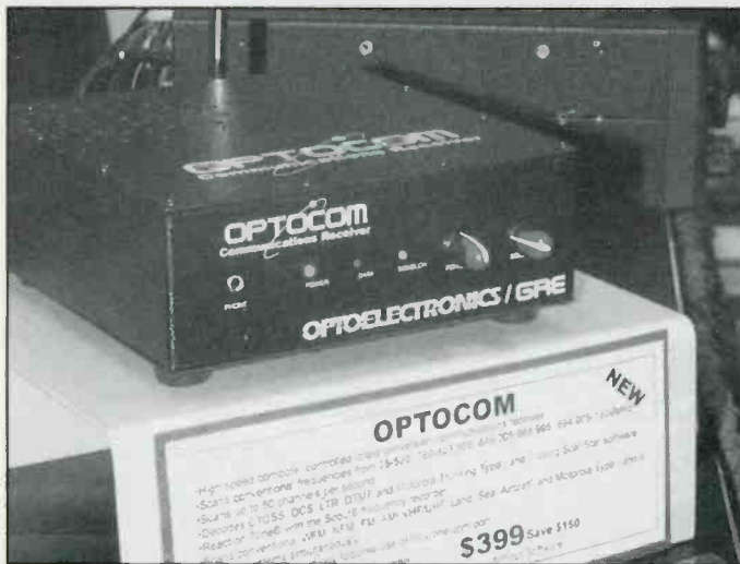
The other exciting product from Optoelectronics is the Optocom, a self-contained black box receiver. It too will follow Johnson LTR and Motorola Type I, II and III trunking with the included version of Trakkstar software from ScanStar. Another exciting feature is the ability to load 28 frequencies or one talk group ID to scan away from the computer.
